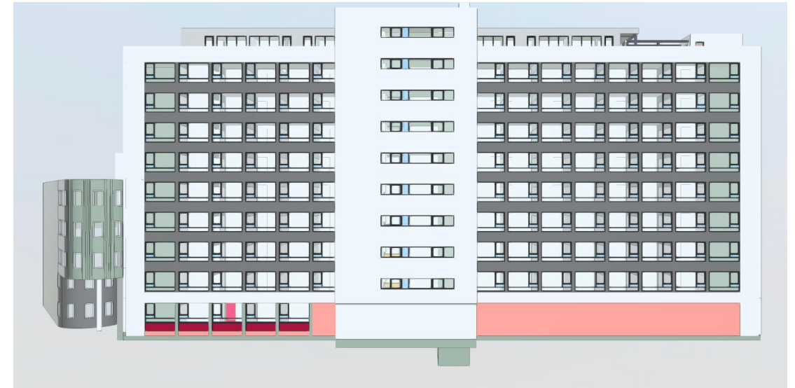
Fig.8 BIM model based on historical blue prints from the 1960s (architectural) [8]
