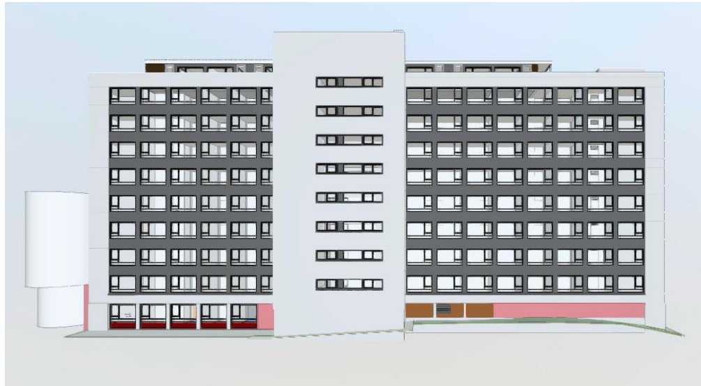
Fig.7 BIM model based on Lidar scans (Pointcloud model) [7]
